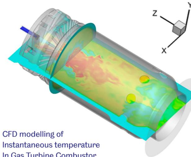
CFD modelling of Instantaneous temperature In Gas Turbine Combustor
